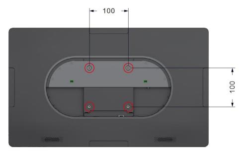
The monitor may be mounted horizontally (output connectors facing down) or vertically (output connectors facing right). Ensure that the surface material and the standard wall mount bracket (purchased separately) are strong enough to support the weight of the monitor (refer to the Specifications table below for weight information).
